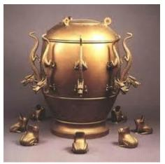
According to court records of the later Han Dynasty, a seismograph was created by the brilliant inventor Zhang Heng (78-140 AD) in 132 AD. Its function is to determine the direction of an earthquake. In 138 AD, this instrument indicated an earthquake occurring in Longxi a thousand kilometers away. It was the first time that mankind to detect an earthquake. Modern seismographs only began development in 1848 in Europe.
